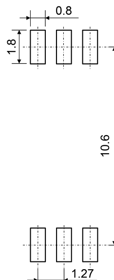
Fig. 15.2 Lead Forming Option (LF4)
